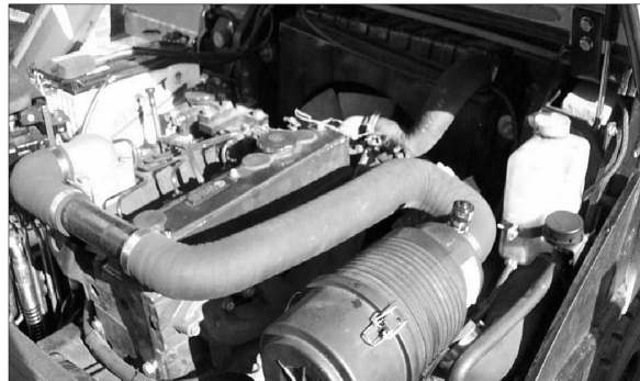
B3.3 Diesel Engine
